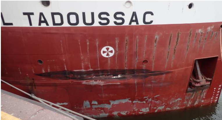
Figure 6. Inside view of damage to the vessel's starboard bow (Source: Canada Steamship Lines)
