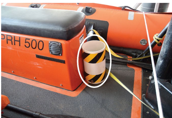
Figure 6. Cylindrical container for brake release line and bag stowage (Source: TSB)
