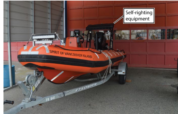
Figure 3. Rescue boat No. 1 with self-righting equipment at the stern (Source: TSB)
