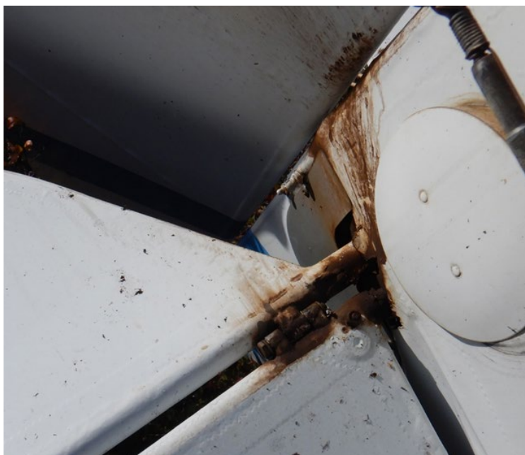
Figure 2. Example of corrosion seen on the occurrence aircraft's tail (Source: TSB)
