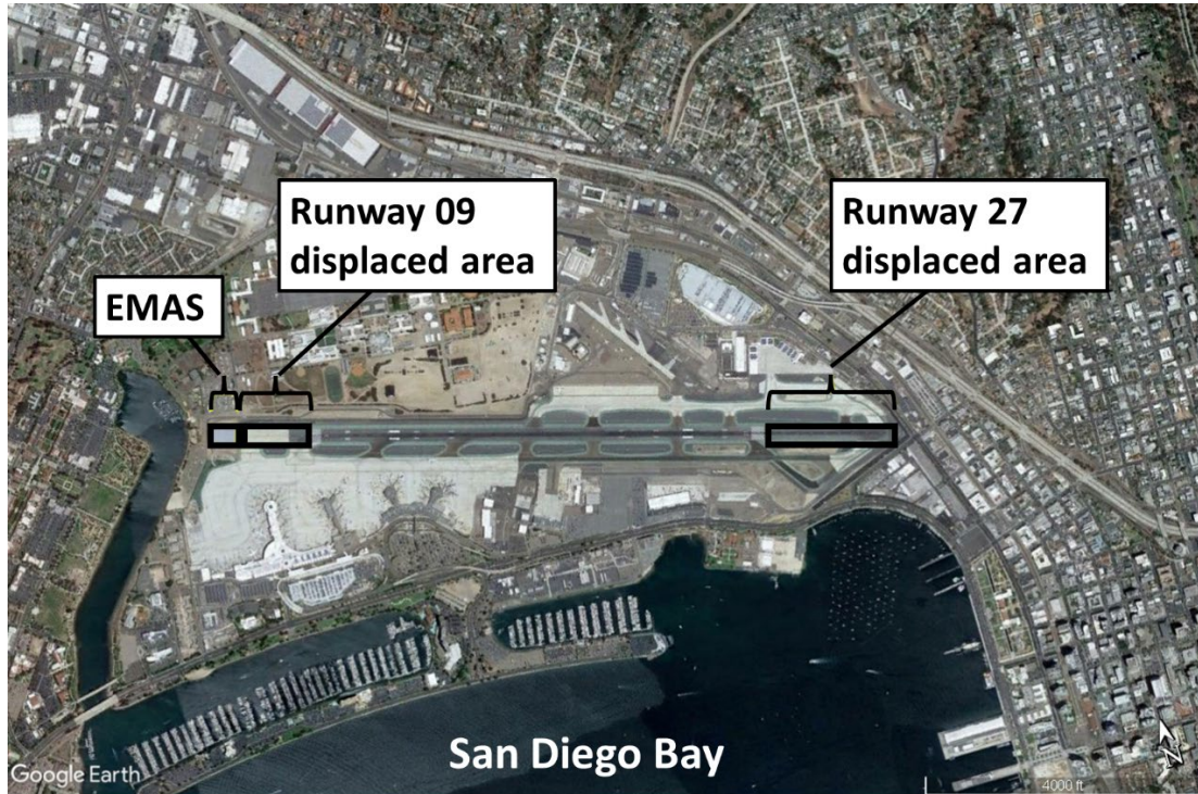
Figure 4. View of San Diego International Airport and Runway 09/27 (Source: Google Earth, with TSB annotations)
