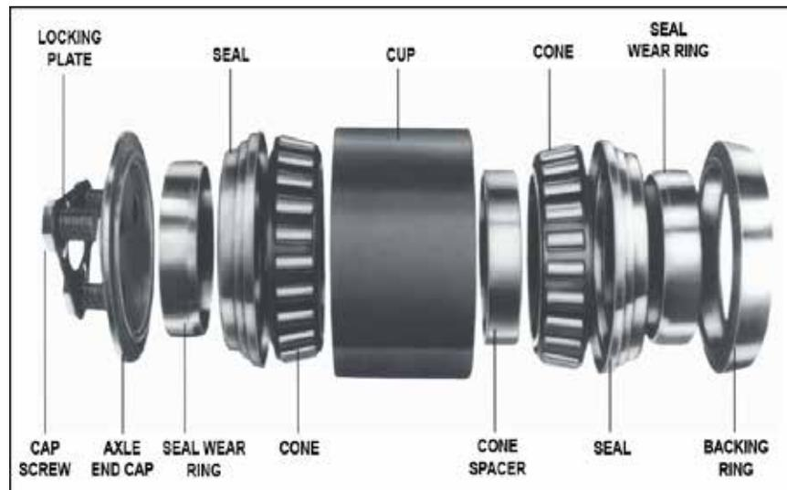
About one million new or reconditioned bearings are mounted each year by North American railways. Roller bearings are designed to last the life of the wheelset without additional lubrication or maintenance. On average, freight car wheelset service life is estimated at
